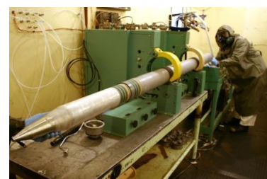
Ammunition Peculiar Equipment (APE) 2097 is used to restrain the shipping and firing tube while the rocket is removed.
